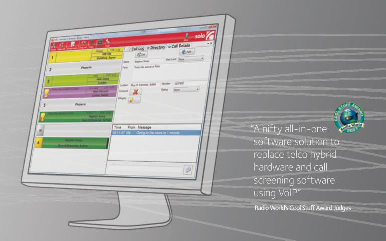
You need very little to get started. Firstly you need some SIP telephone lines. These can come directly from your existing office switch if it can supply SIP extensions, alternatively a conversion gateway can be purchased to convert your existing analogue or ISDN lines to SIP. Secondly, you need a soundcard. (Ask for recommended brands). Thirdly you need a SIP handset (Ask for recommended brands.) Lastly, your PC.
